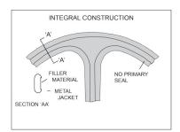
If leakage occurs across the pass partition bar, the fluid will flow along the length of the pass bar arrangements, and then flow to the outer diameter of the gasket being retained only by the secondary seal. The intermediate part of the gasket does very little to effect the sealing capabilities of the gasket.
