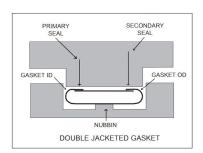
Due to the high bolt loads required to seat metal jacketed gaskets, designers often incorporate stress raising nubbins on the flange sealing face, the principle being that the majority of the applied bolt load is acting on a relatively small proportion of the gasket surface area, thus high surface stresses result. It is essential that the gasket is installed with the smooth side toward the nubbin.
