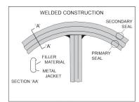
With a welded pass bar arrangement the fluid is retained by the primary seal at the inner diameter of the gasket. Thus the primary seal maintains its function, providing a seal of higher integrity.
